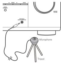
If you have a tripod, use it to place the microphone so that it's about ear level at your normal listening position. Otherwise, place the microphone at ear level using a table or a chair.
